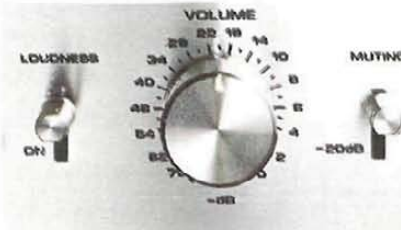
Click-stop volume control calibrated in decibels, with left/right tracking within 0.5 dB.
