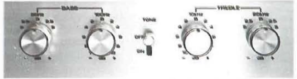
Twin tone-control system with step-type settings, permitting 3025 possible combinations.
